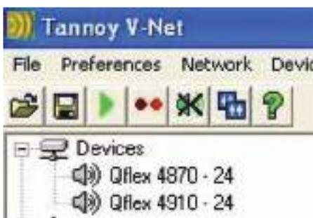
If PodWare becomes unable to communicate with a device for some reason whilst on-line (such as a break in the network cable), the corresponding icon for it in the Devices node of the Tree will appear in red, indicating that control and monitoring on that device is invalid. Most devices will allow themselves to be 'rediscovered' automatically if such a cable break is repaired.
