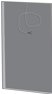
Fig. 3. Drywall Cutout with Speaker Cable
