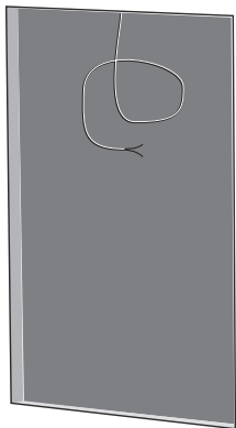
Fig. 3. Drywall Cutout with Speaker Cable
