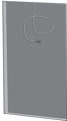
Fig. 3. Drywall Cutout with Speaker Cable
