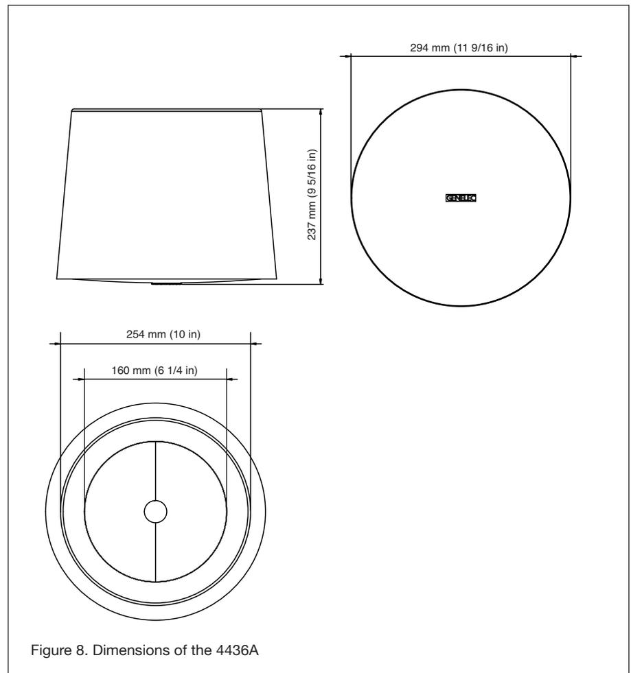
Figure 8. Dimensions of the 4436A
