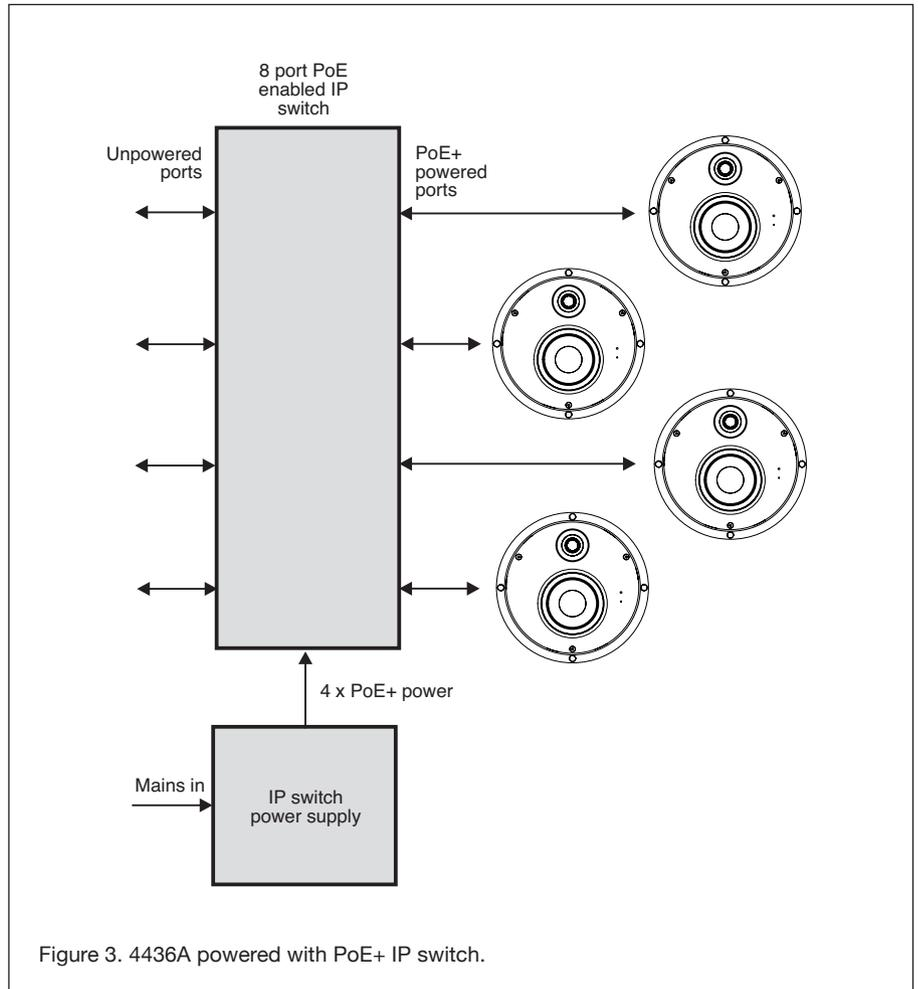
Figure 3. 4436A powered with PoE+ IP switch.
