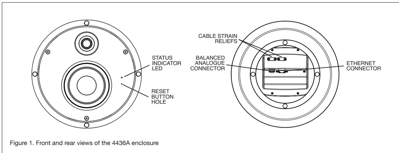
Figure 1. Front and rear views of the 4436A enclosure
