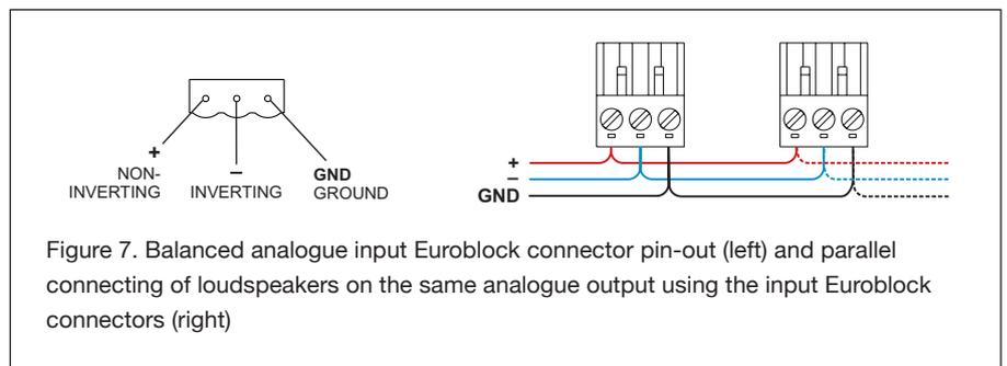
Figure 7. Balanced analogue input Euroblock connector pin-out (left) and parallel connecting of loudspeakers on the same analogue output using the input Euroblock connectors (right)
