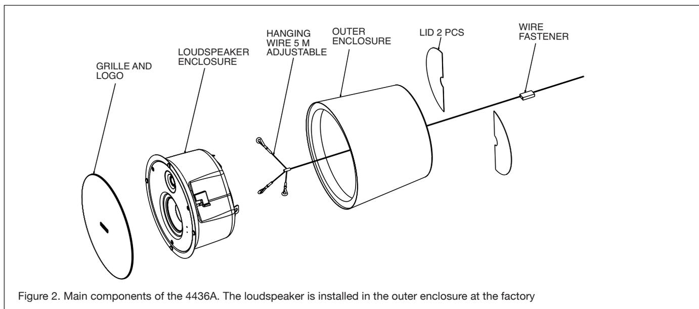
Figure 2. Main components of the 4436A. The loudspeaker is installed in the outer enclosure at the factory
