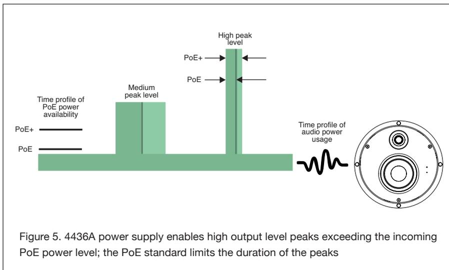
Figure 5. 4436A power supply enables high output level peaks exceeding the incoming PoE power level; the PoE standard limits the duration of the peaks
