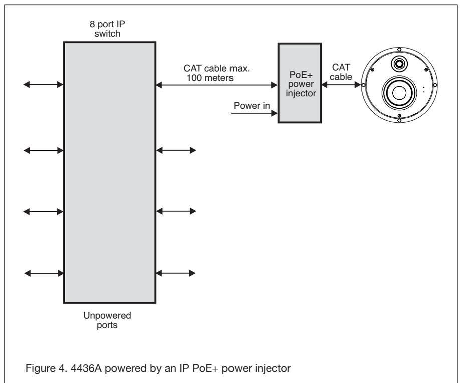
Figure 4. 4436A powered by an IP PoE+ power injector
