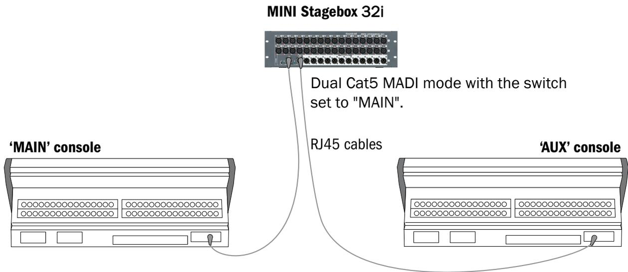
This console will control preamp gain and will be able to access the Mini Stagebox outputs.
