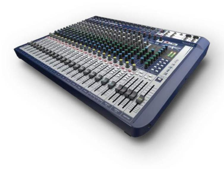
Input channels take sources and route/process them. The sources catered for by the Signature consoles includes mono (single channel) sources, stereo sources, and internal sources (the FX Return channel).
