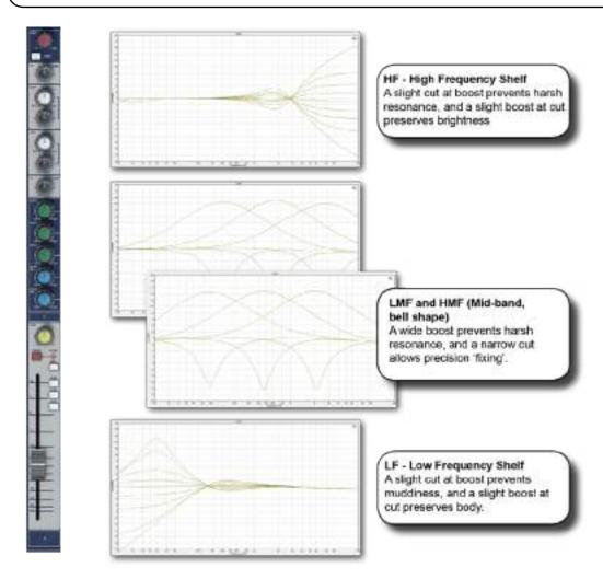
The shelving bands of the EQ (LF and HF) use a slight boost at the EQ's frequency when cutting, and a slight cut when boosting.
