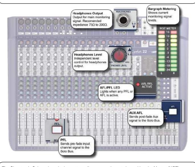
The Signature's Solo and monitoring system allows an engineer to hear either the Master (MST) stereo outputs or any channels currently assigned to the Solo bus, via the headphone output.
