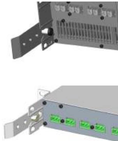
Figure 6.3: Rear support bracket mounted for removable installation and bracket pointing towards rear
