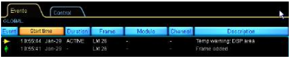
Figure 17-3: Global Events Warning Indication
